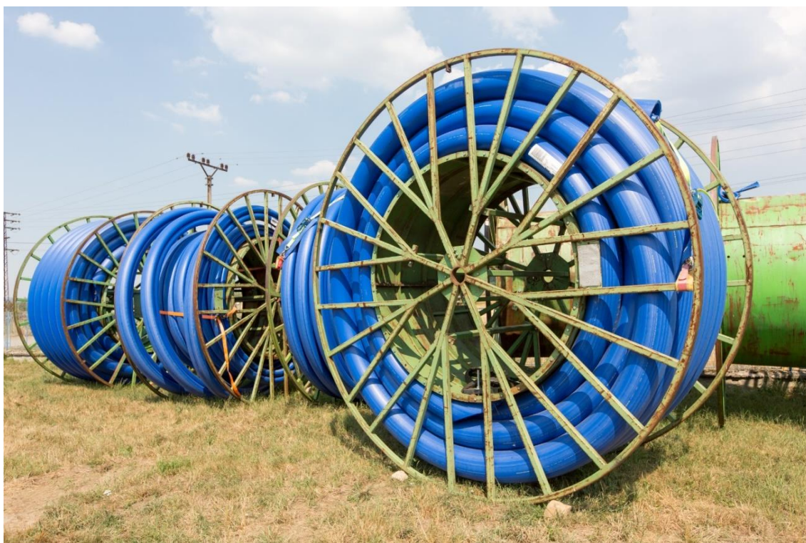
Obr. 4 Bubny s navinutou trubkou Compact Pipe DN350
